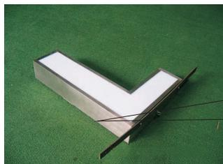
Double sides illuminating letter. The depth of the letter should be less than 60mm; Recommended length for series connection is not more than 5m; Parallel connection recommended between several strips
